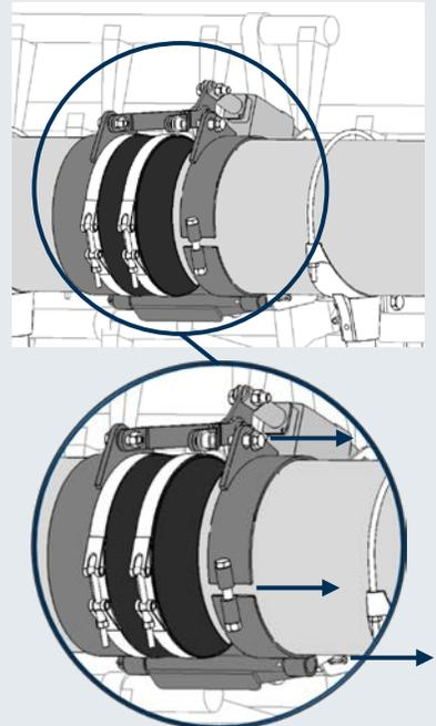
8. With a person at each end of the manifold, lift center pivot end and rotate to disengage lock sleeve bushing.
