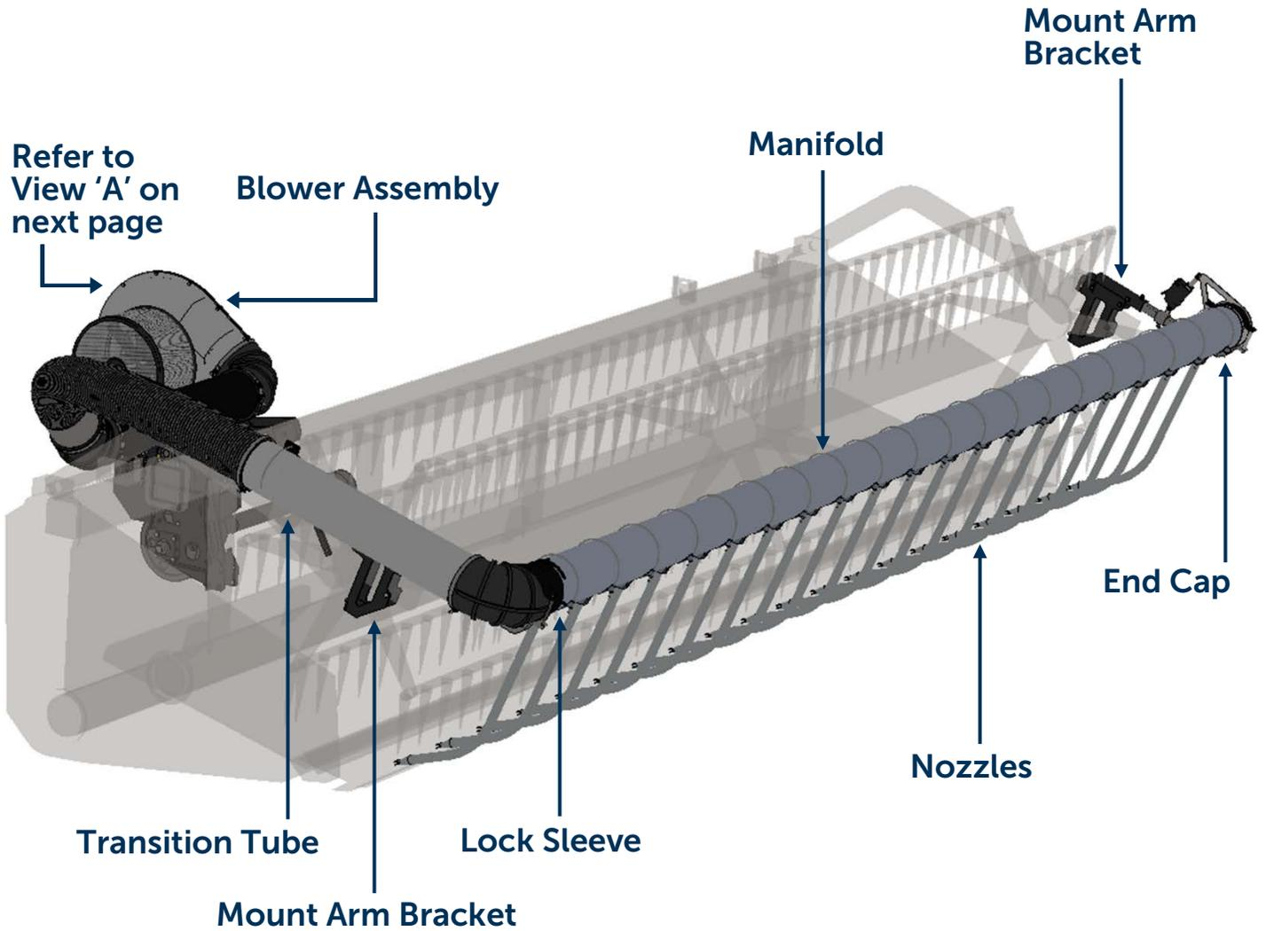
**Manifold Tilt Mechanism
